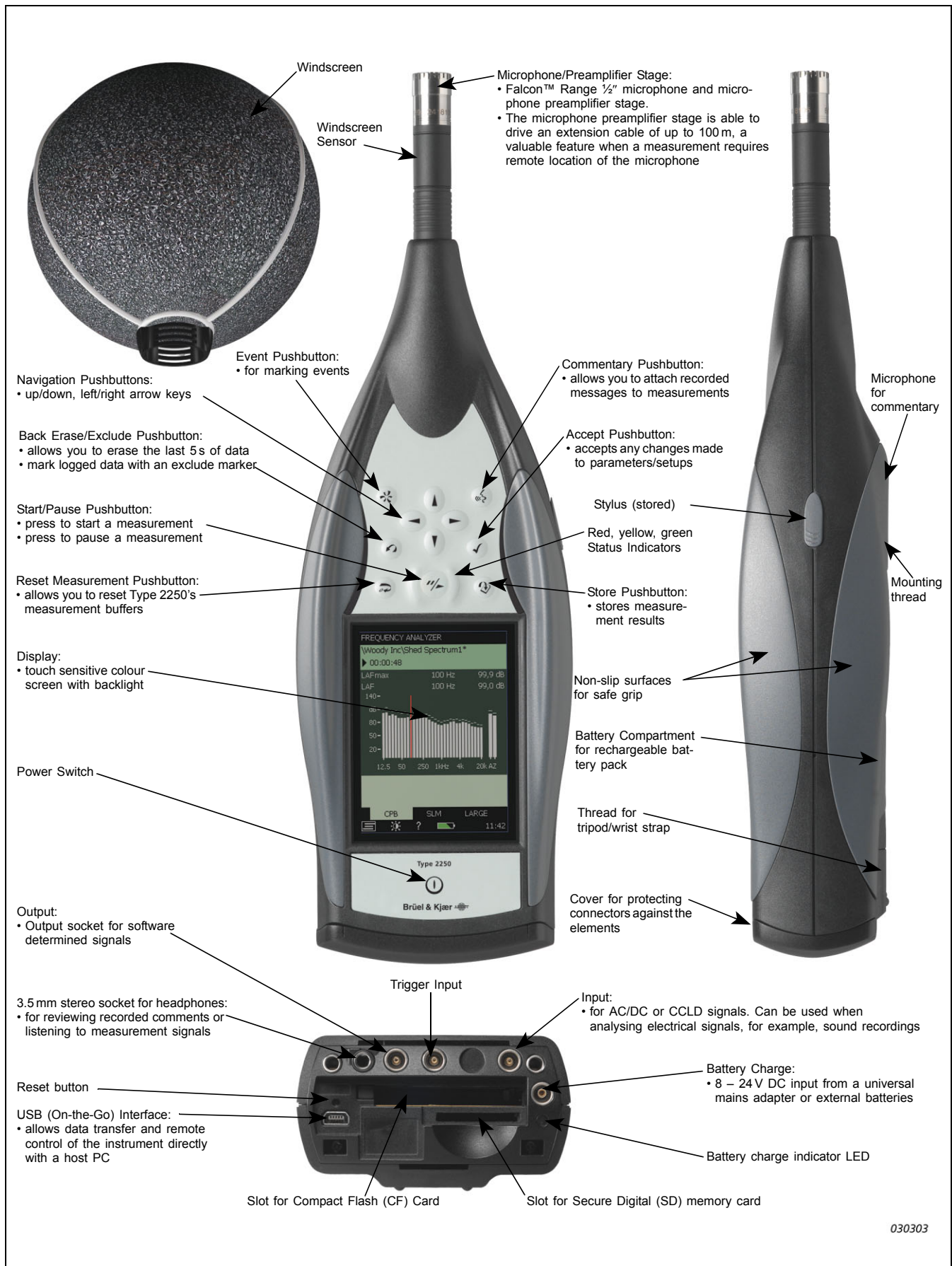
Fig. 1 Key features of Hand-held Analyzer Type 2250
